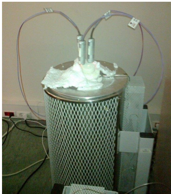
Work with constructed Au/Pt thermocouples at TUBITAK UME, annealing of Au/Pt
