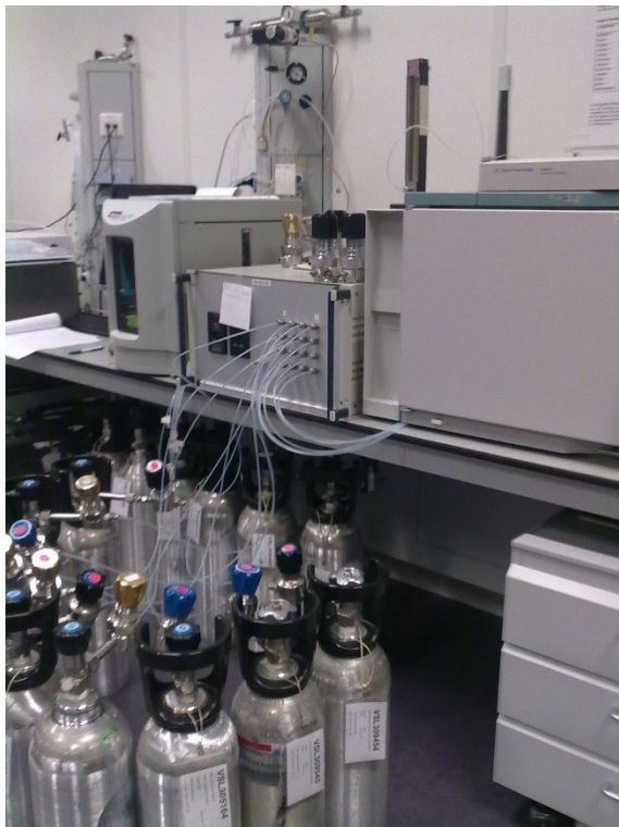
Gas Chromatograph with FID and TCD detectors for the analysis of the components of natural gas mixtures
