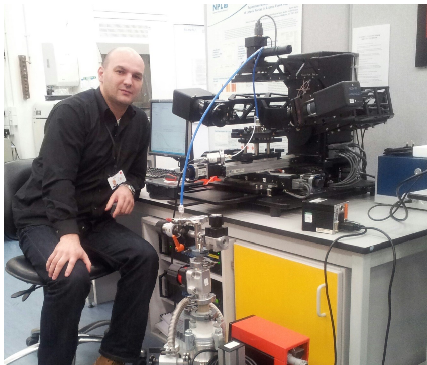
Testing of material surface of weight standard- ellipsometry
