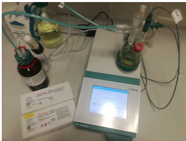
Fischer coulometer used for purity assessment of ethanol
