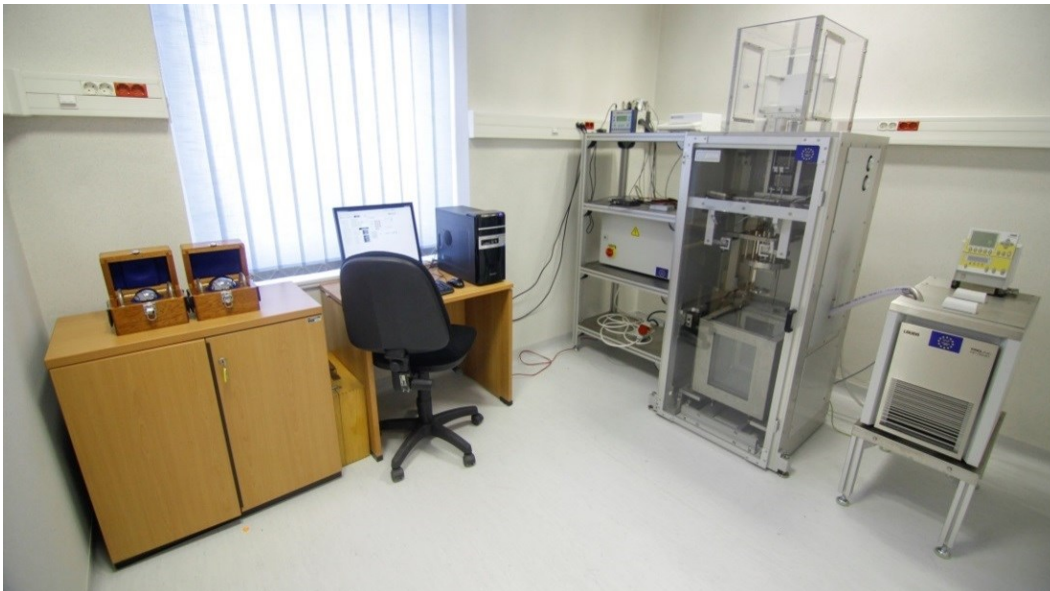
Hydrostatic weighing instrument for primary realization of liquid density in LM IMBILH
