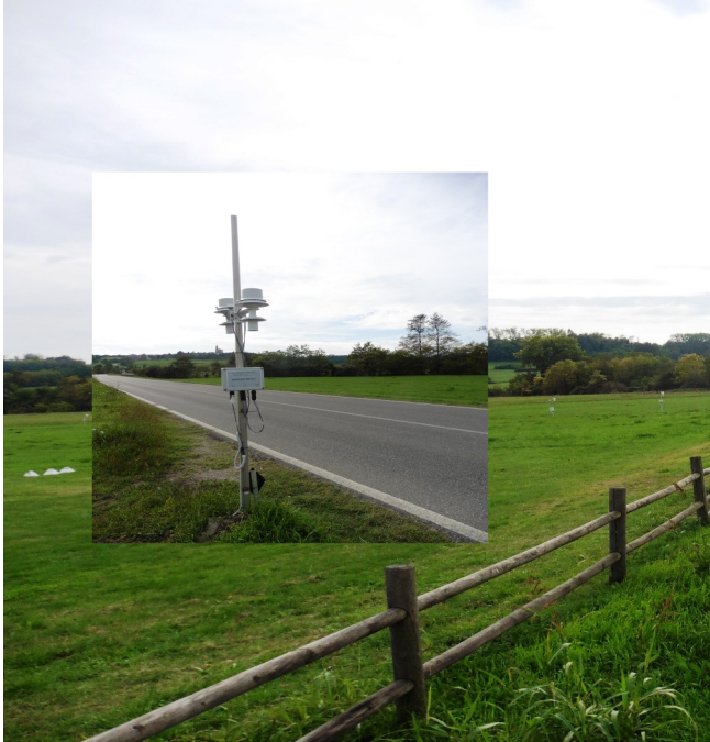
Experimental setup for the evaluation of obstacles on land ground based air temperature measurements
